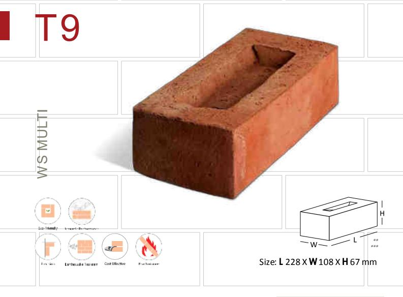
A traditional brick having a very unique molding process believed to have originated in England and is called the "Water Struck" process wherin a very high moisture content day is pressed into molds. Water is the lubricant used to release the wet day from the molds. The resultant towelling of the wet day by the mold box as the wet bricks slide
